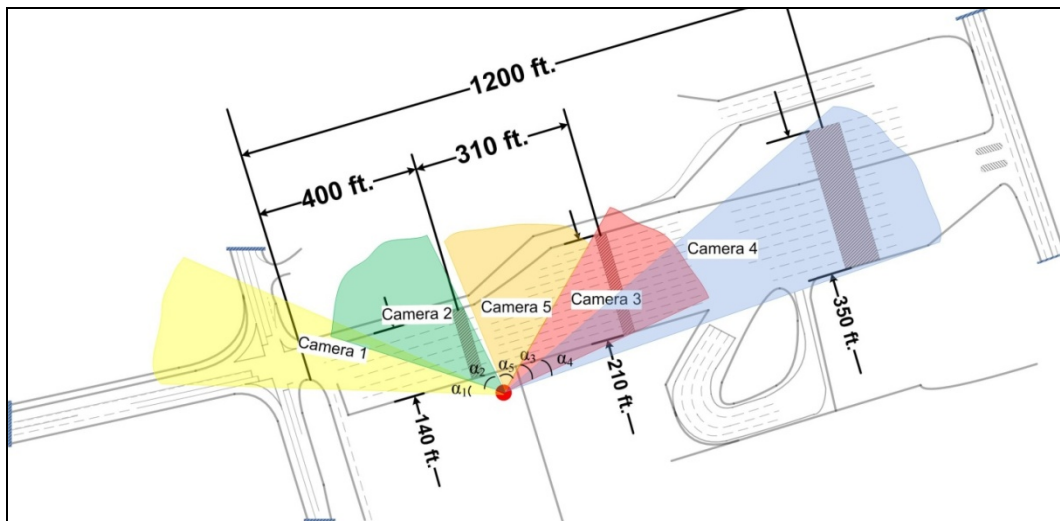
Figure 4.7 Camera configurations for the proposed vision-based sensing system
